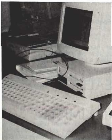
Apricot's new F2 model — 512 K of RAM, twin 720 K 3.5 inch disk drives, a mouse and GEM for £1495 (NZ$3750)
